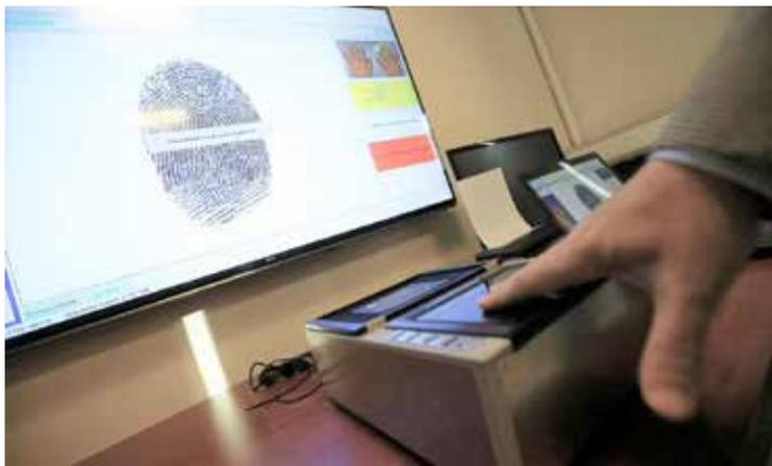
The fingerprint scanners integrated into the unit check the person's identity within seconds and ensure the accuracy of the information provided by the subject. Unlike many standard scanners in the sector that clip the print for the sake of query and matching speed, Papilon scanners offer speed and accuracy in one package without clipping the print.
