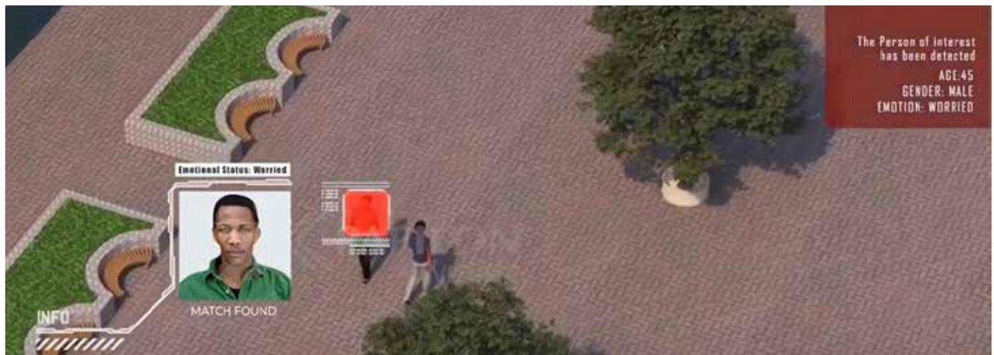
The system works in integration with Papilon's central biometric data management and storage systems Polyface or APFIS and instantly compares facial images captured with the UAV's camera with those held in the systems' datasets. The system compares the photographs of citizens taken for official procedures and the real time footage from the vehicular camera. The system then looks for matches and authenticates the identity of the subject.
